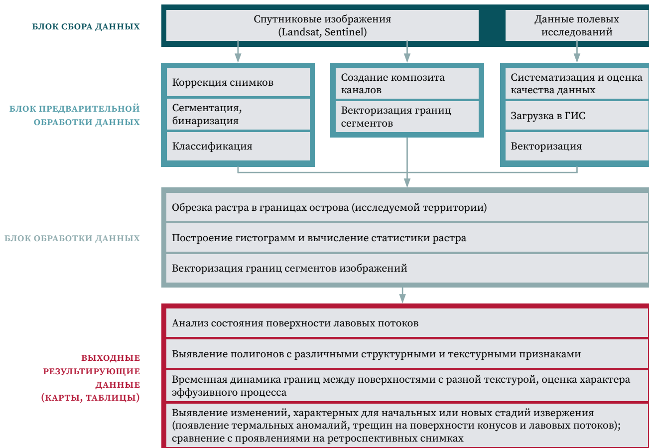
Fig. 1 Technological scheme of preparation and processing of materials for monitoring territories exposed to effusive volcanoes (according to [6] with changes)
